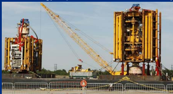
Blow out Preventer & Lower Marine Riser Pack
